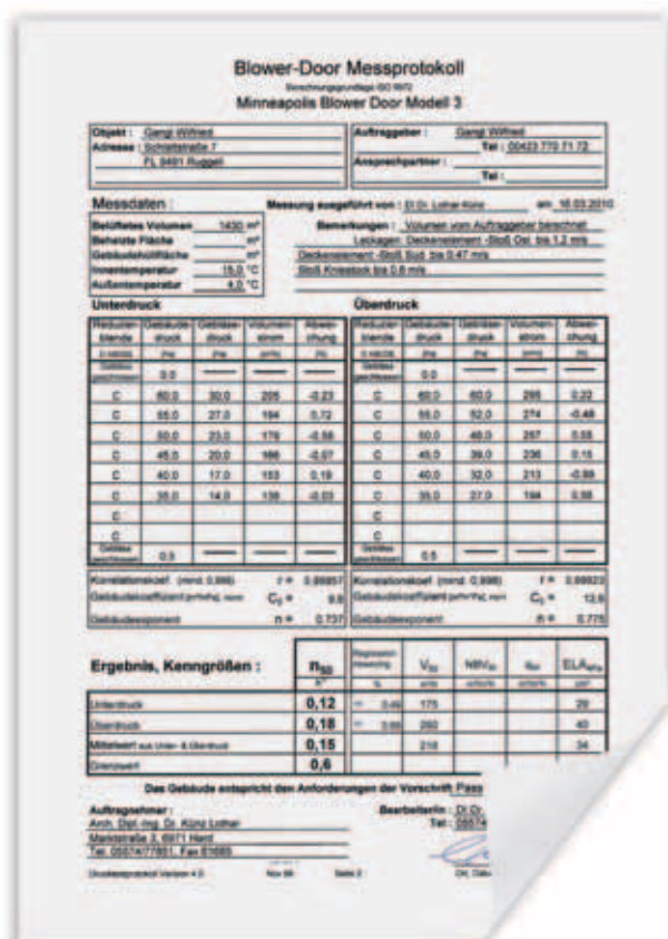
Fig. 9: A Blower Door Test in a passive house built with KLH solid wood panels. Through the support of an excellent air tightness concept, an n_{50} -value of 0,15 \text{ h}^{-1} could be realised [with the kind support of Eberle • d e n k f a b r i k • Dornbirn, Austria].
